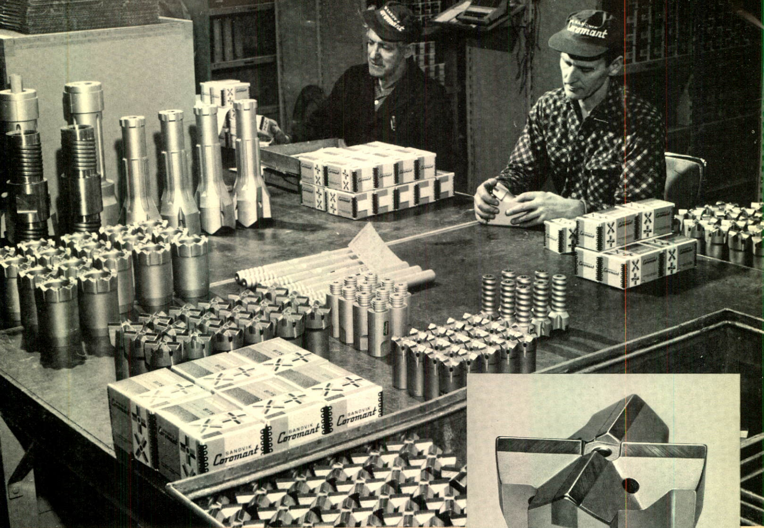
Packing various types of Coromant detachable drill bits tipped with tungsten carbide.
