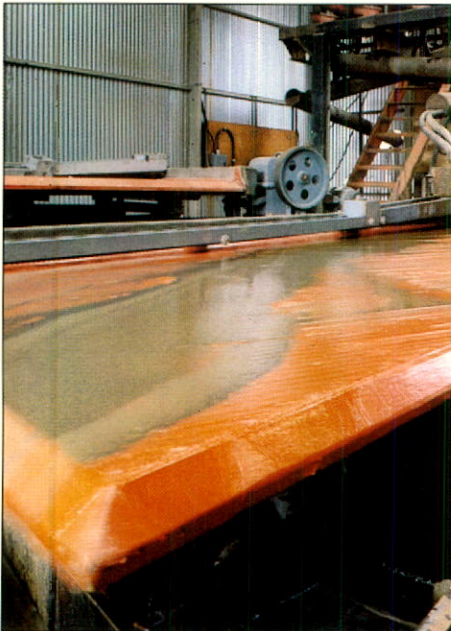
ABOVE: Spiral and table concentration equipment at Dublin Gulch placer operation.
