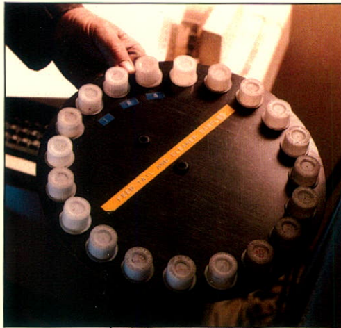
Samples are prepared for X-ray analysis during each shift, to assist process control.
