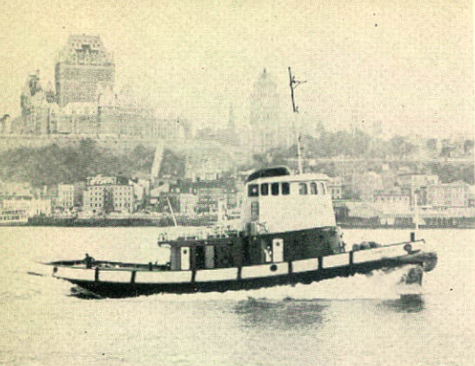
"Charlie S" — Modern Davie-operated diesel tug. Constructed 1954 in 55 working days.
