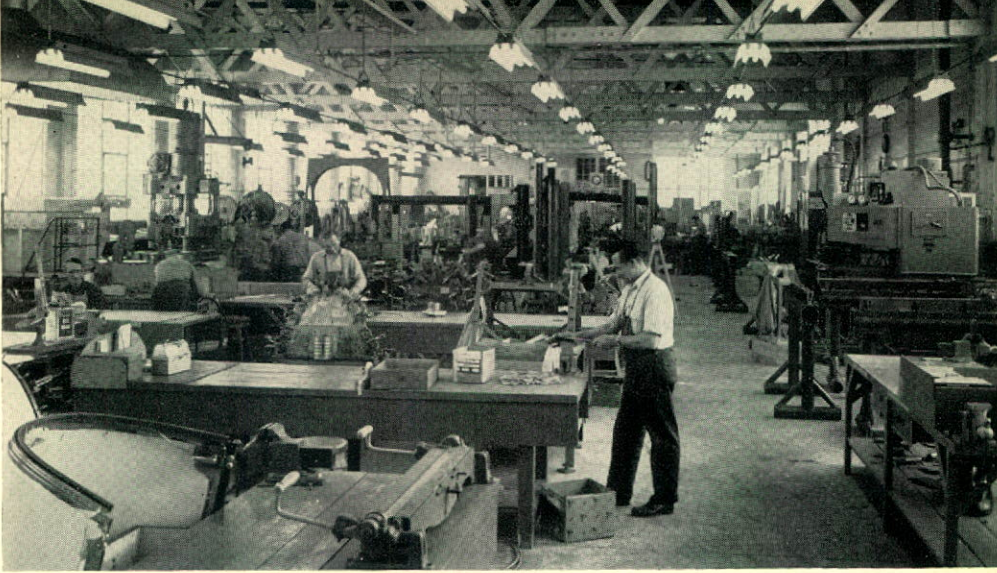
Interior view of the aircraft shop, showing canopies and sub-assemblies for wing details under construction for Beech, Harvard and de Havilland aircraft. This work is typical of the varied activities performed by the Port Arthur Shipbuilding Company for Canadian industry.
