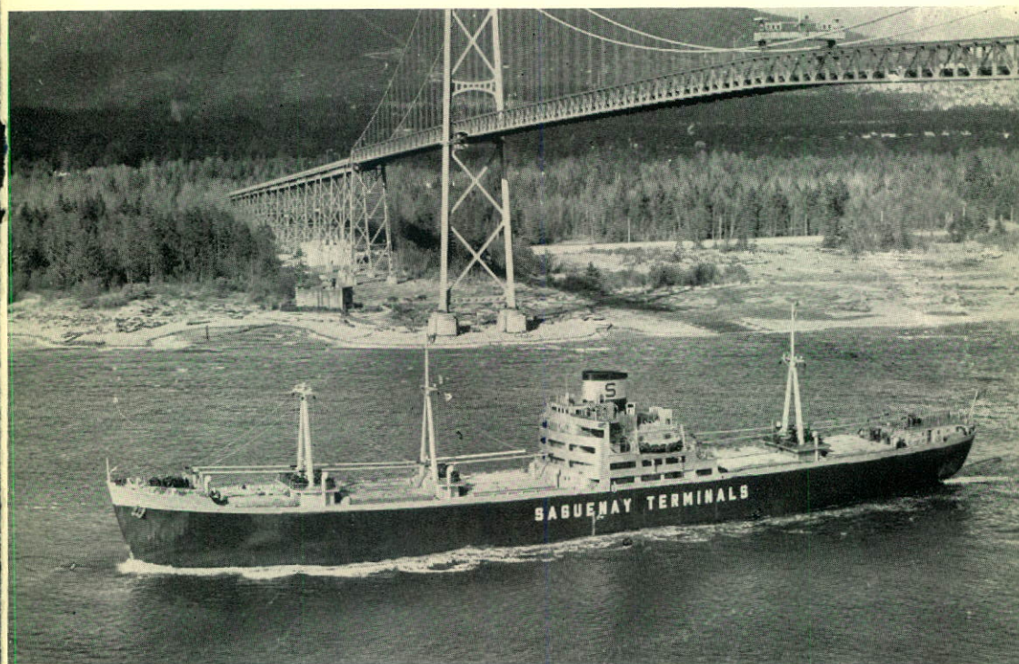
The S.S. "SUNRIP" — designed and built for Saguenay Terminals by Davie — was the first ship in the world to have an all-welded aluminum superstructure.
