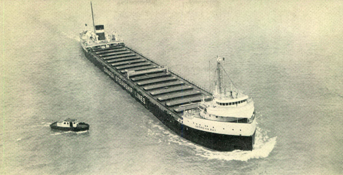
The S.S. GEORGIAN BAY — a C.S.L. Upper Lake bulk freighter, constructed at Collingwood Shipyard.
