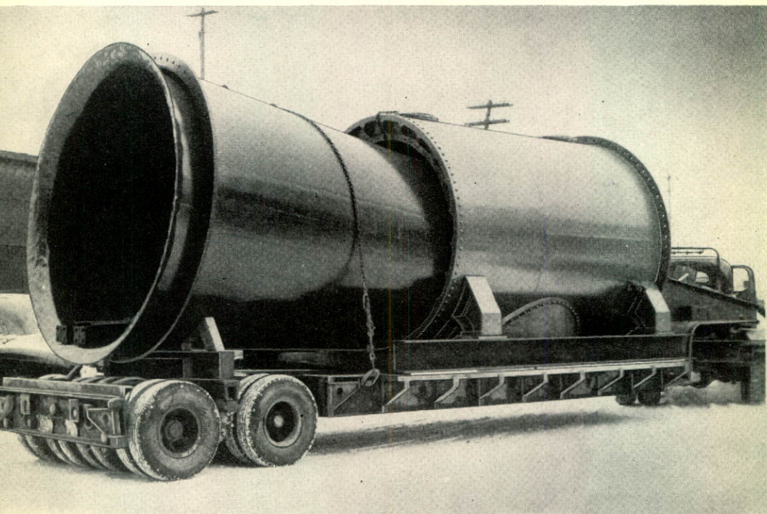
Giant draft tube and turbine casing produced at Collingwood.
