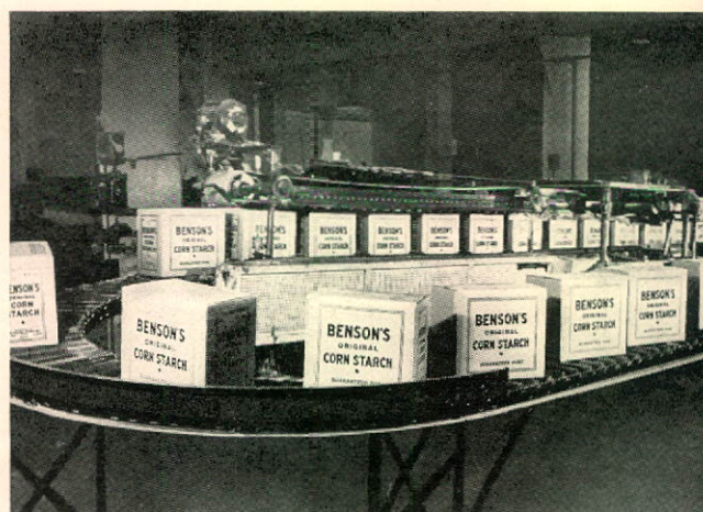
The completed shipping cases proceed to Finished Goods warehouse after being sealed on an automatic case sealer.
