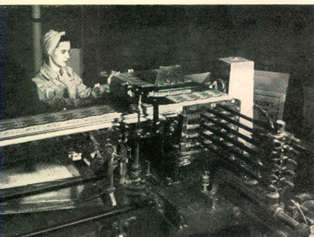
The cartons then move to the completely automatic case filler where they are packed 40 units to the container.
