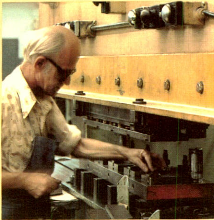
Howard McGuin forms metal components on a heavy duty press.
