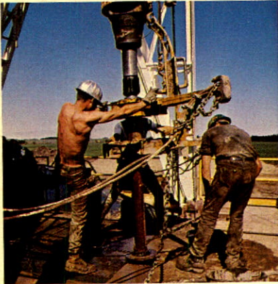
Drilling crew preparing to pull pipe
