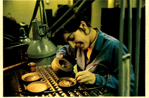
Wesdrill technician setting diamond drilling bits
