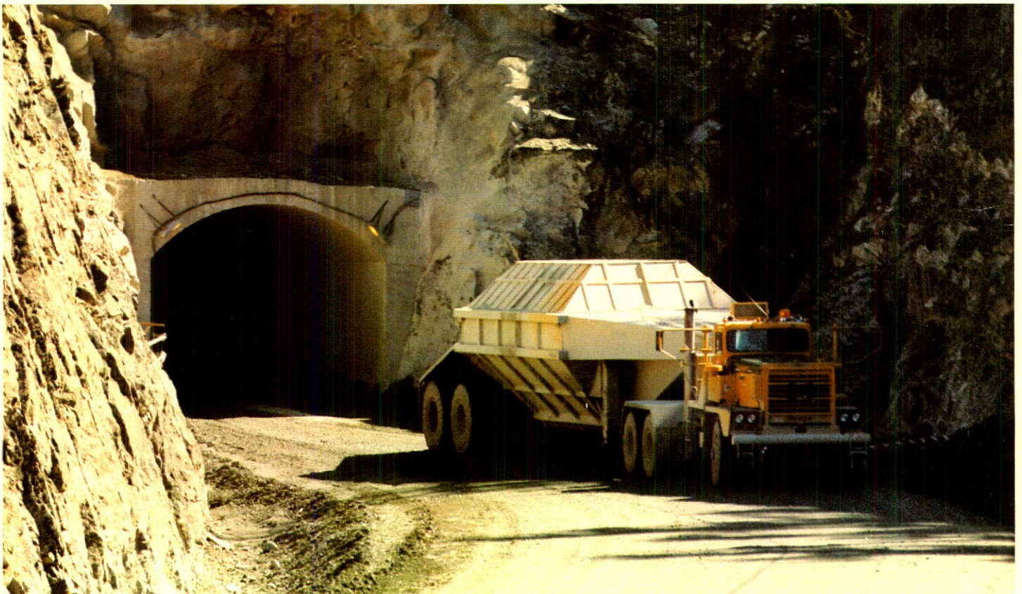
Thetford Mines, Québec — one of six trucks, each of 110-ton capacity, transporting ore from the King-Beaver pit via a 900-foot rock tunnel to the Normandie mill.
