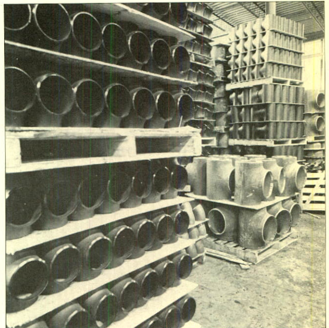
Welding fittings in CCTF warehouse.
